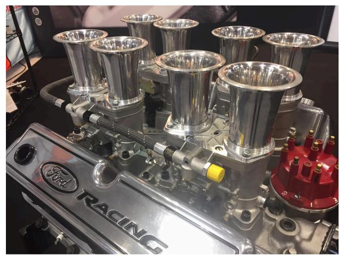
The Jenvey Heritage IDF throttle body comes in TDFQ45 and TDFQ48 mm bore options. This is a single twin throttle body set up to suit 8 cylinder engines.
