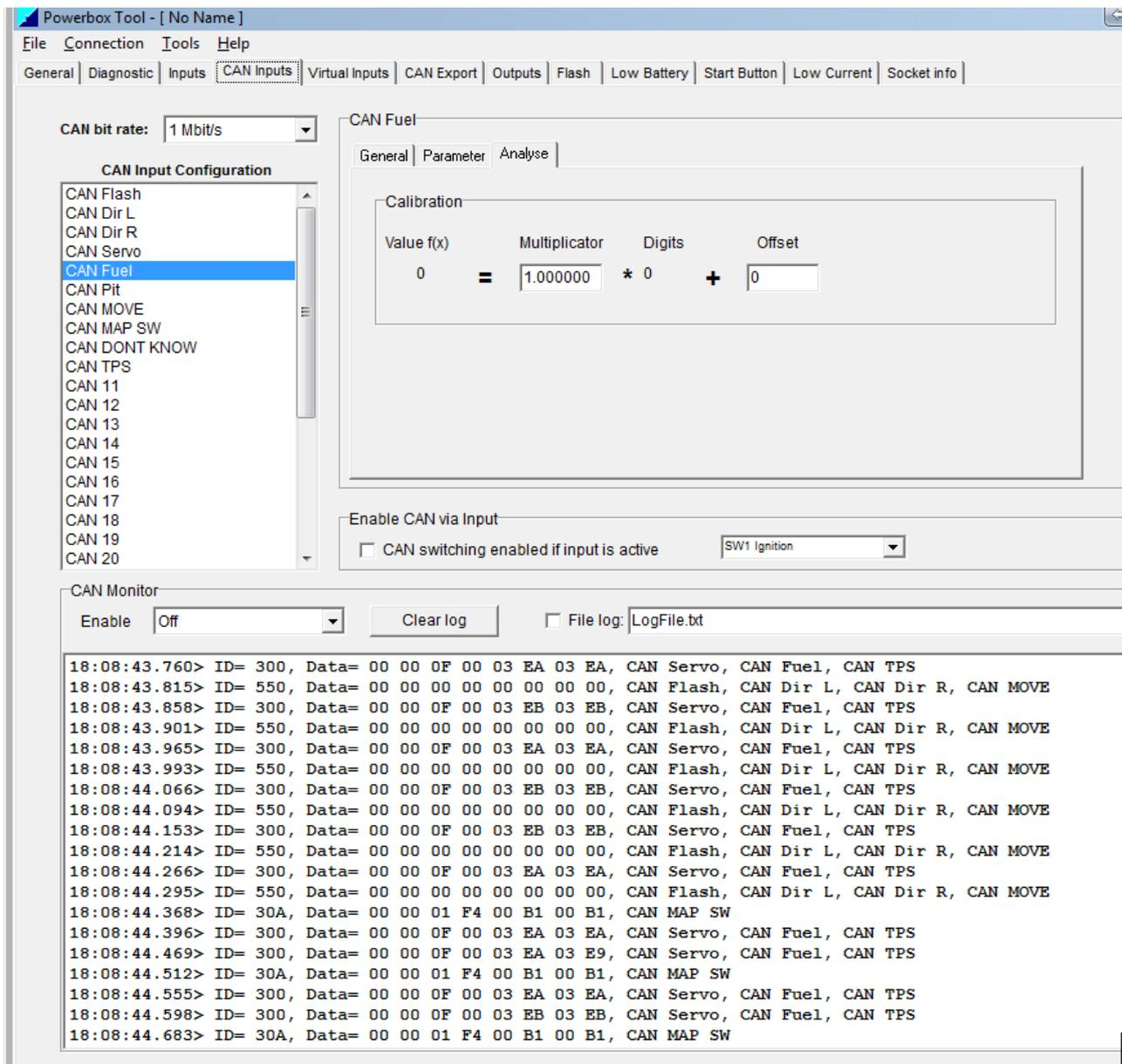
The Software can show the CAN traffic in the CAN Monitor window, it is possible to select between different filters, this helps to analyze the CAN traffic, a log to file function is also possible.
