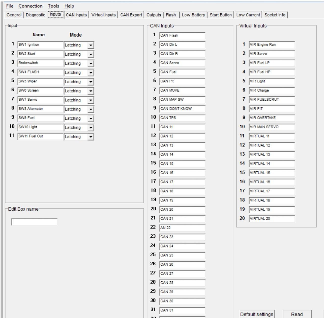
The conventional inputs are digital channels. The standard configuration of the PCM only accepts connections switching to ground (except Switch #1 which has to switch to battery voltage to activate), either to enable or to disable a channel.
