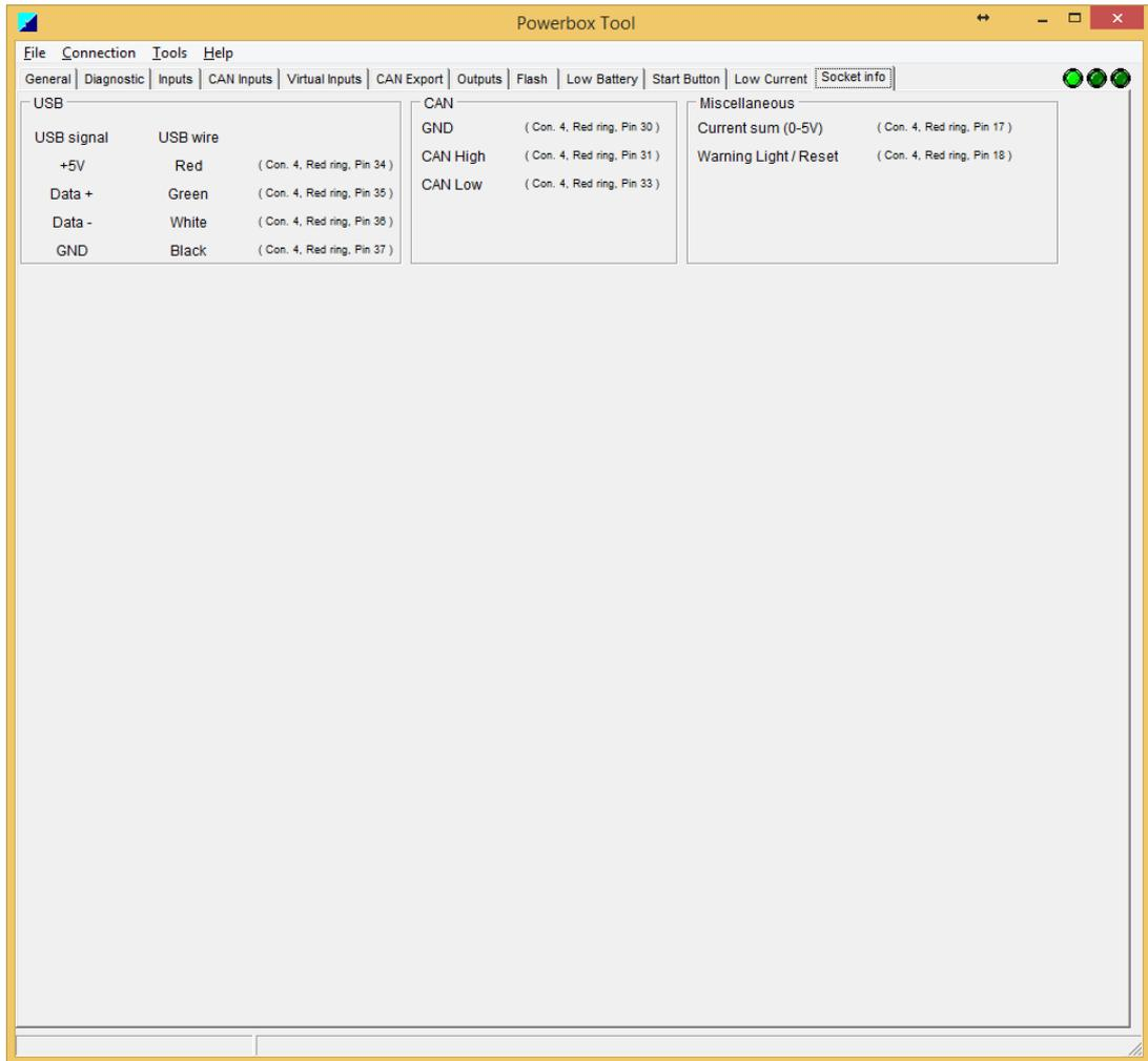
This window explains the pin out of the USB, CAN and Miscellaneous functions.
