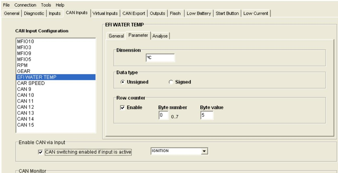
Bytes are read as unsigned by default. This means that data is read in bits from 0..255, 0..1023 or 0..65535.
