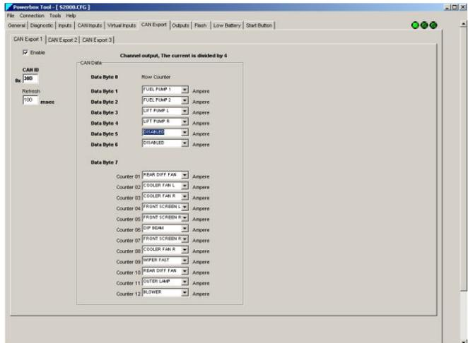
Type the number of channels rotating in byte 7 in the **Row Count** window.
