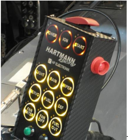
The panel is equipped with 12 buttons, each button has two functions - Momentary and Toggle. - NEW! Now you have also a possibility to make 2 stages on your output, first push A next B third off, or/and A, A+B and off. Also we are now supporting Can speed 500Kbit and 1Mbit - Please see Technical Manual V.2 -
